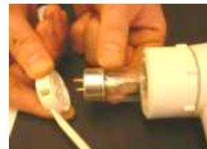
5). Disconnect lamp holders and remove lamp
